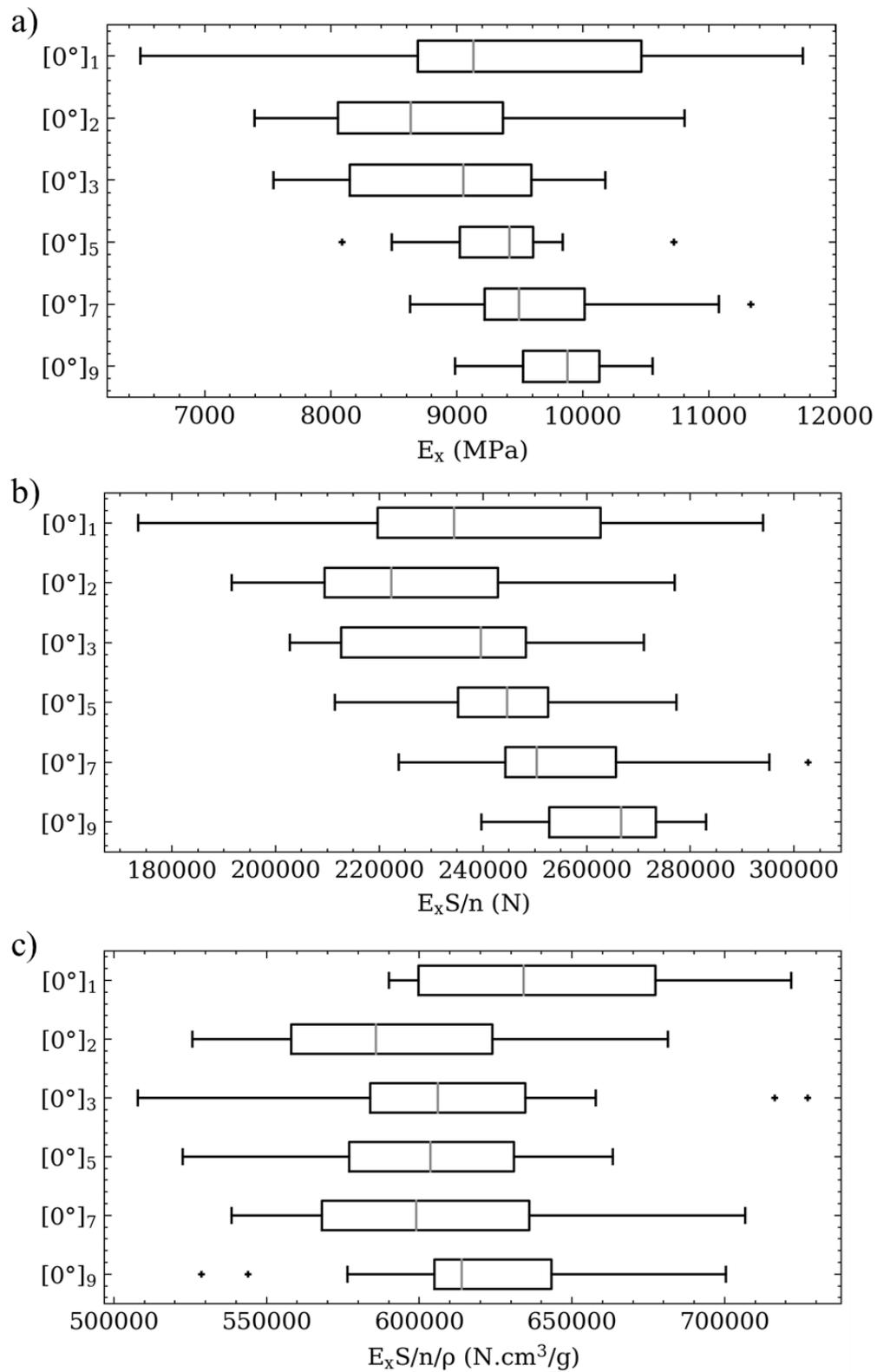
**Figure 1.** Distribution of the longitudinal Young's modulus by series (a), the Young's modulus multiplied by the cross-section and relative to the number of plies (b), and the specific Young's modulus multiplied by the cross-section and related to the number of plies (c)
