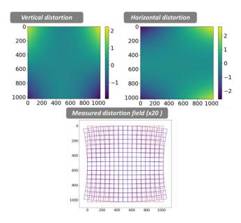
Figure 3: Evaluation of the lens distortion using digital image correlation on the overlap regions of the image mosaic. Vertical and horizontal distortion functions, illustration of the magnified measured distortion field (x20)
