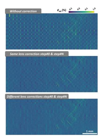
Figure 2: Influence of the lens distortion correction of the strain map of the whole region of interest at the onset of microplasticity: No correction, correction using the distortion function from the reference images, correction using the distortion function for each loading step.
