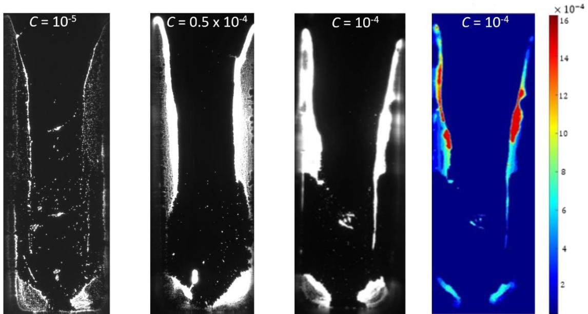
**Fig. 9.** Spatial distribution of deposited particles at the end of experiment after full evaporation. The preferential zones of particle deposition are in bright. The false color image on the right shows a more detailed information on the deposited particle distribution for the highest concentration tested.
