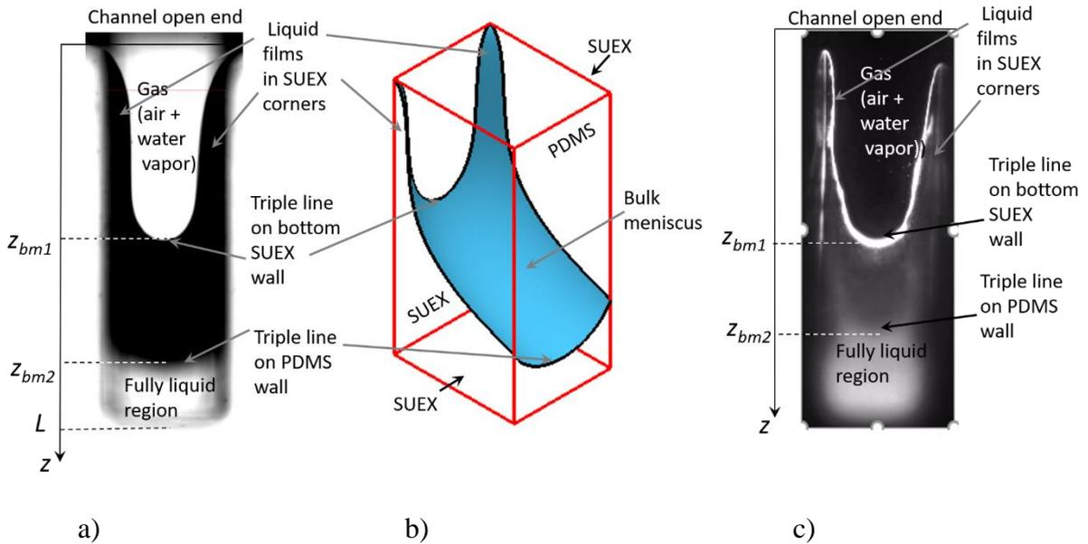
**Fig. 3.** Typical fluid distribution in the channel during evaporation: a) top view of the channel in the experiment with pure water, b) quasi-static shape computed with Surface Evolver for  $\theta_{SUEX} = 30^\circ$  and  $\theta_{PDMS} = 104^\circ$ , c) in the presence of particles ( $C = 10^{-4}$  g/mL)
