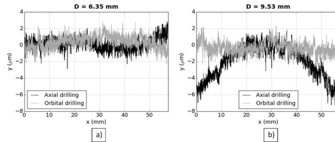
**Fig. 10.** Specimen deformation profiles obtained with the HOCT.
