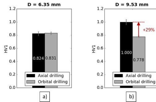
**Fig. 7.** Normalized microhardness results (as a ratio of the maximum value).
