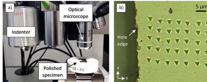
**Fig. 3.** (a) Nanoindentation device. (b) Matrix of indents obtained.
