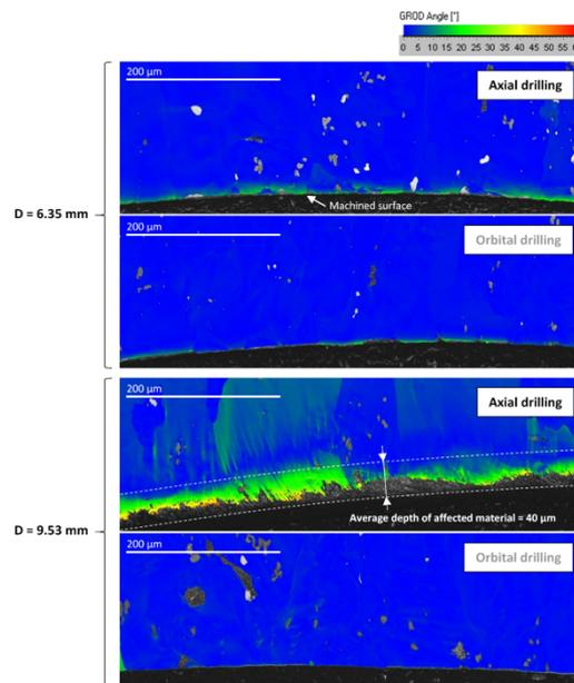
**Fig. 9.** GROD mapping in the hole edge area.
