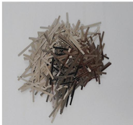
**Figure 2.** 30 mm-long metallic fibres.
