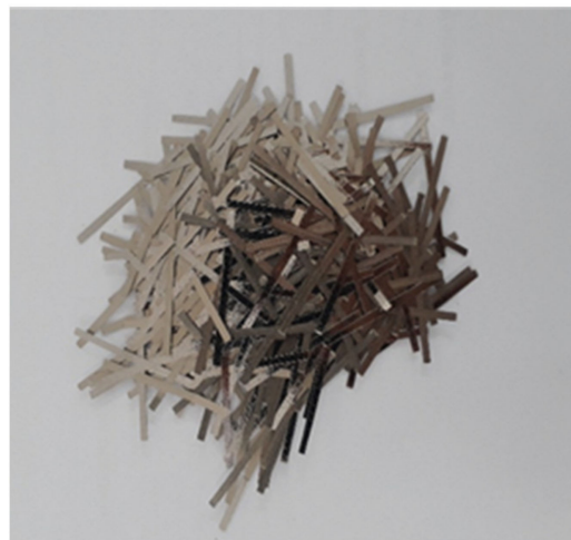
Figure 2. 30 mm-long metallic fibres.
