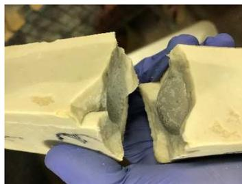
Figure 12: A grout bar of formulation S16-B6.5, broken after passing 90 days in Na<sub>2</sub>SO<sub>4</sub> solution at SO<sub>3</sub> concentration of 3000 mg/L.
