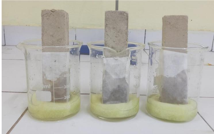
**Figure 6: Capillary water absorption of an adobe**
