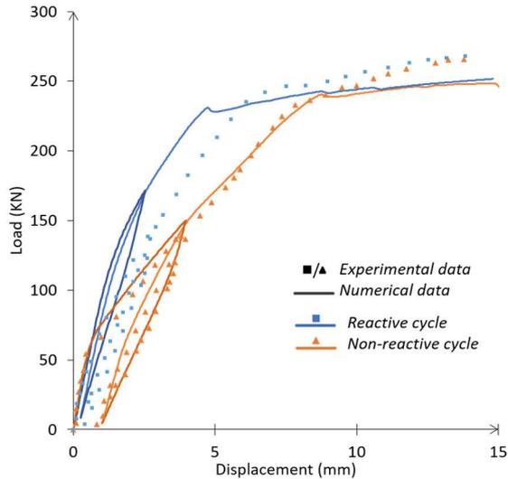
Figure 12 : 17 month load-displacement curves with a cyclic load
