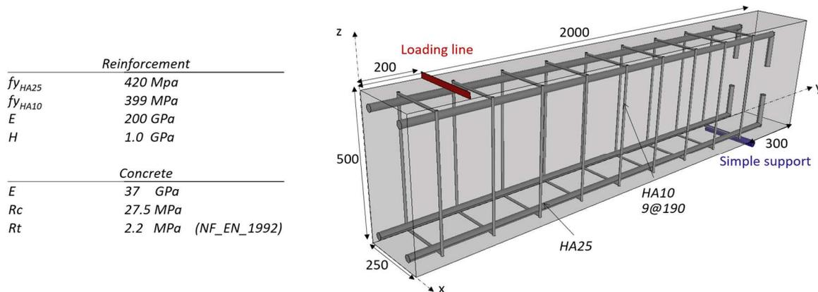
315 *Figure 3 : Mechanical characteristics and half-beam reinforcement (unit = mm)*
