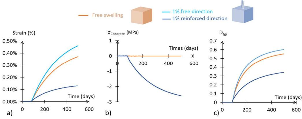
Figure 2: Effect of reinforcement compared to stress-free swelling, a) Strain evolution, b) Concrete stress evolution, c) ASR-damage evolution
