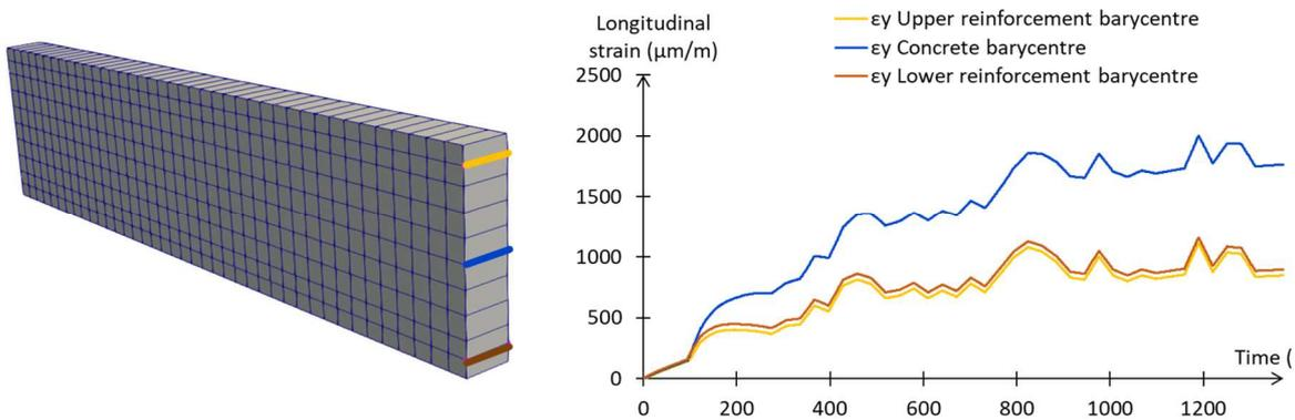
Figure 8 : Strain evolution between the reinforcements and concrete barycentre
