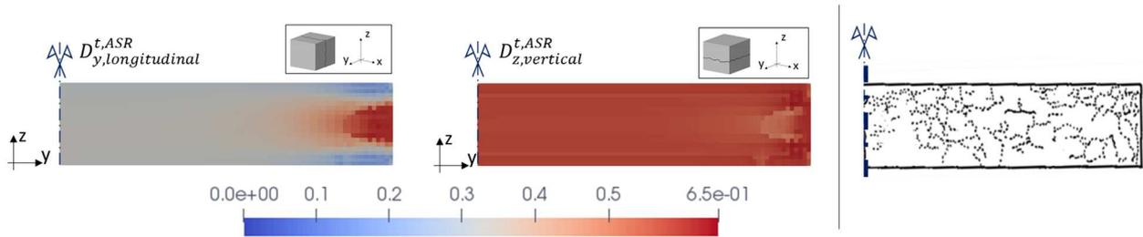
Figure 9 : Anisotropic swelling damage for the 45 month case
