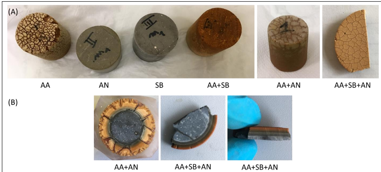
206 Figure 2: (A) Visual appearance of the samples' surfaces at the end of the experiment and (B) visual appearance of the slices 207 of the samples AA+AN and AA+SB+AN at the end of the experiment (AA: acetic acid, AN: ammonium nitrate, SB: sodium 208 bicarbonate)
