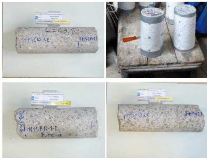
245 246 Fig. 2. Cores extracted from Song Loulou dam for the LPC N° 44 test, credit to Guedon - 247 IFSTTAR 2010
