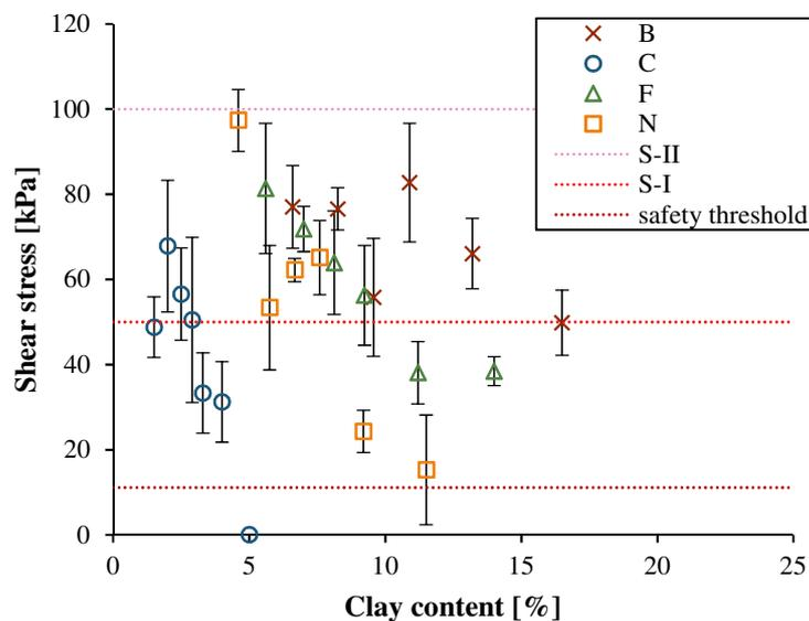
**Figure 15.** Shear stress of unstabilized plasters.
