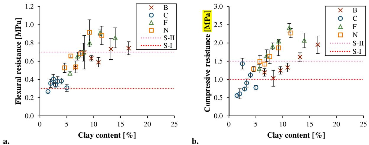
**Figure 13.** (a.) Flexural and (b.) compressive resistances of prismatic specimens of mortars depending on their clay contents.
