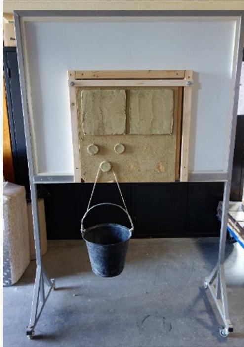
**Figure 3.** Shear test assembly.
