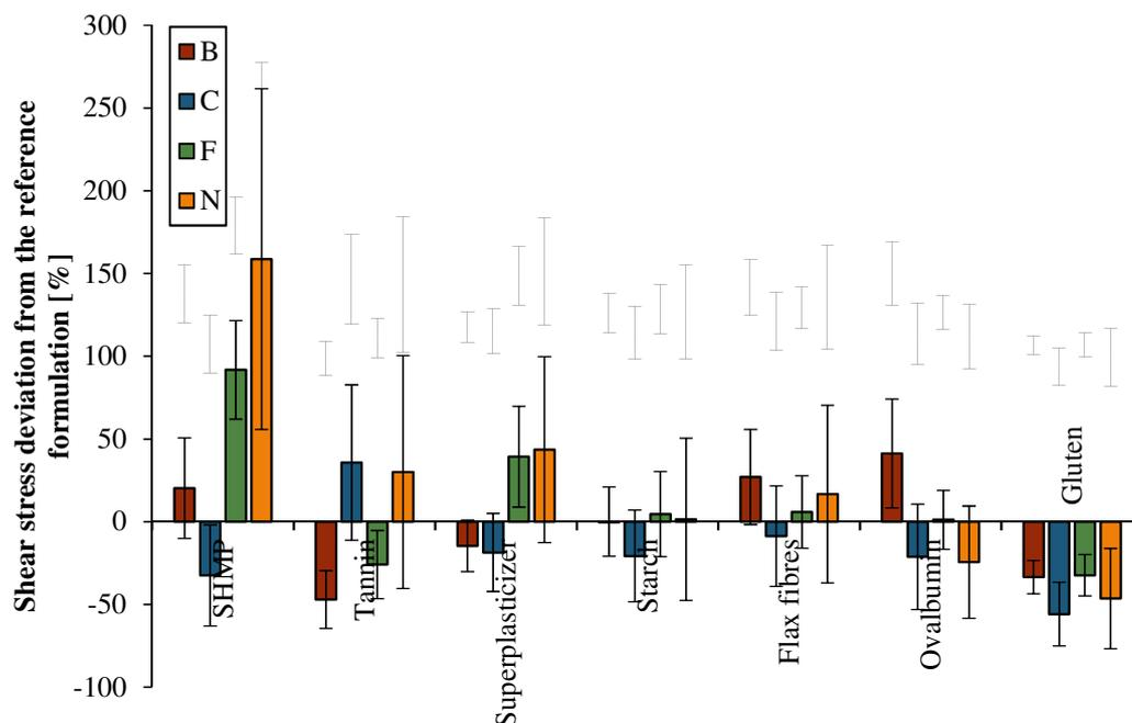
**Figure 16.** Effect of admixtures on shear stress.
