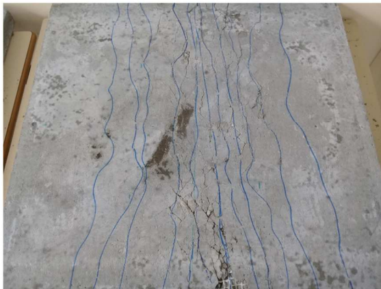
10wt% PCM-TRC (3,70 cm crack spacing)
