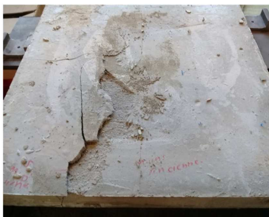
Compression crushing failure 10wt% PCM-TRC slab at 20°C
