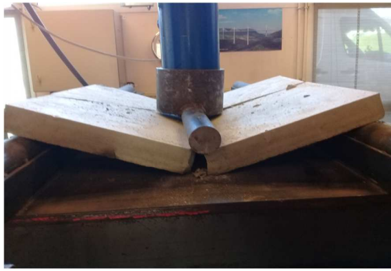
Brittle behaviour of unreinforced TRC slab
