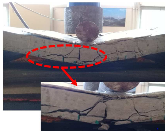
Delamination failure 10wt% PCM-TRC slab at 40°C
