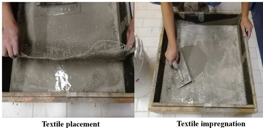
A- Insitu hand lay-up technique
