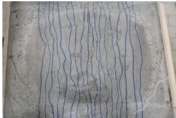
Ductile and multicracking behaviour of reinforced TRC slab
