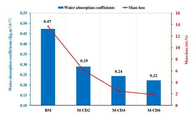
Fig. 9. Water absorption coefficients and mass loss of earth renders versus cow dung contents
