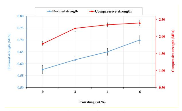
Fig. 12. Flexural and compressive strengths of earth rendering mortars reinforced by cow dung
