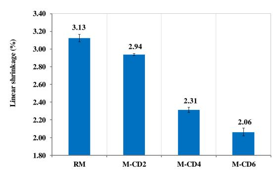
Fig. 7. Linear shrinkage of earth rendering mortars according to cow dung content
