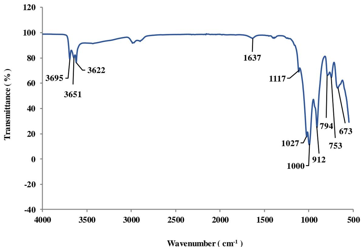
**Fig. 3. FTIR spectrum of the raw material**
