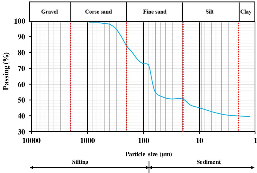
**Fig. 1. Particle size distribution of the soil**
