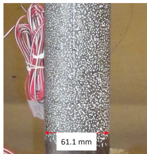
Figure 11. Random pattern on the surface of the thick composite tube [16].
