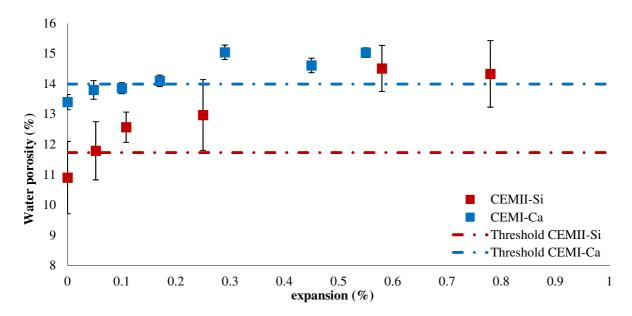
Figure 13: Evolution of water porosity as a function of expansion for concretes damaged by
