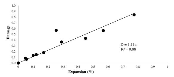
Figure 18: Evolution of the damage as a function of expansion
