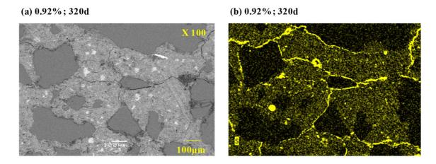
Figure 8: CEMII-Si SEM images (a) initial image and (b) sulfur image (mapping)
