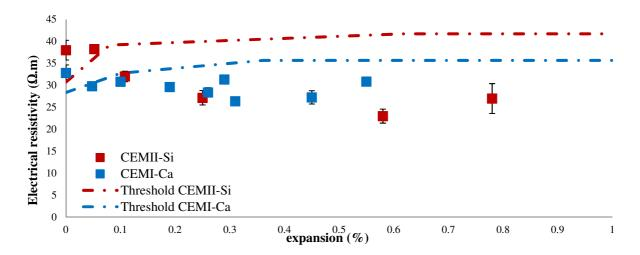
Figure 12: Evolution of the coefficient of the electrical resistivity according to the expansion for concretes damaged by DEF
