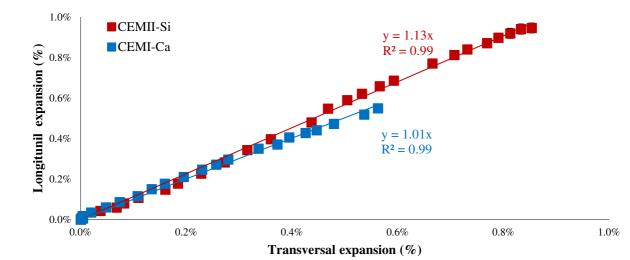
Figure 5: Evolution of longitudinal vs. transversal expansion
