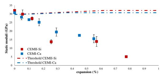
Figure 16: Evolution of the static moduli according to the expansion for concretes damaged by DEF
