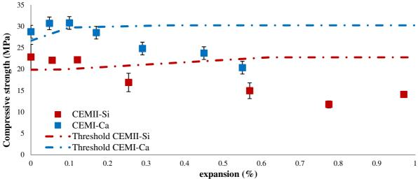
Figure 15: Evolution of the compressive strength according to the expansion for concretes damaged by DEF
