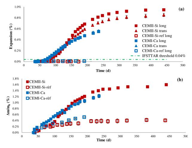
Figure 4: Evolution of expansion (transversal and longitudinal) (a) and mass gain (b) versus
