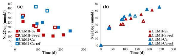
Figure 10: Evolution of the equivalent alkali content in the interstitial solution (a) and in the storage water (b) versus time
