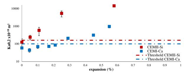
Figure 14: Evolution of apparent gas permeability coefficient according to the expansion for concretes damaged by DEF
