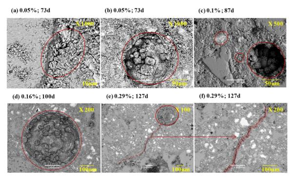
Figure 7: SEM images of the CEMI-Ca concrete
