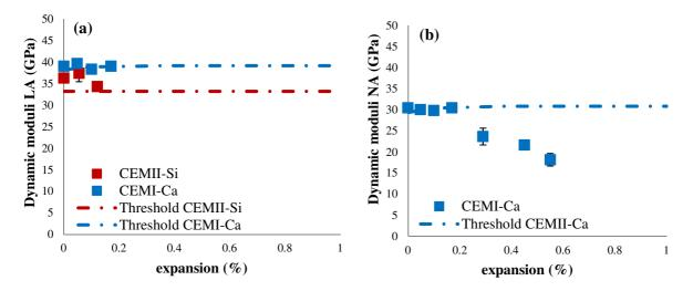
Figure 17: Evolution of the dynamic moduli in linear (a) and nonlinear (b) acoustics
