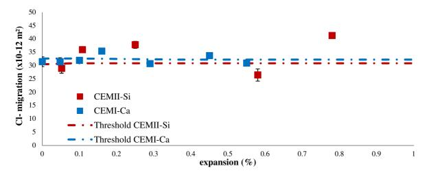
Figure 11: Evolution of the coefficient of migration of chlorine ions according to the expansion for concretes damaged by DEF
