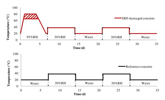
Figure 1: Thermal profile of concretes developing DEF and wet/dry cycles for both concretes
