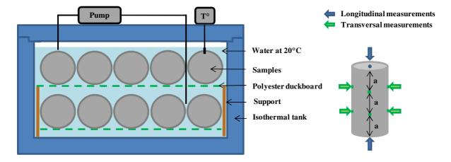
Figure 2: Sample storage and measurements of dimensions
