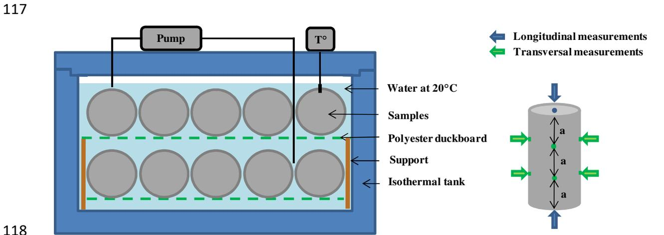
119 Figure 2: Sample storage and measurements of dimensions
