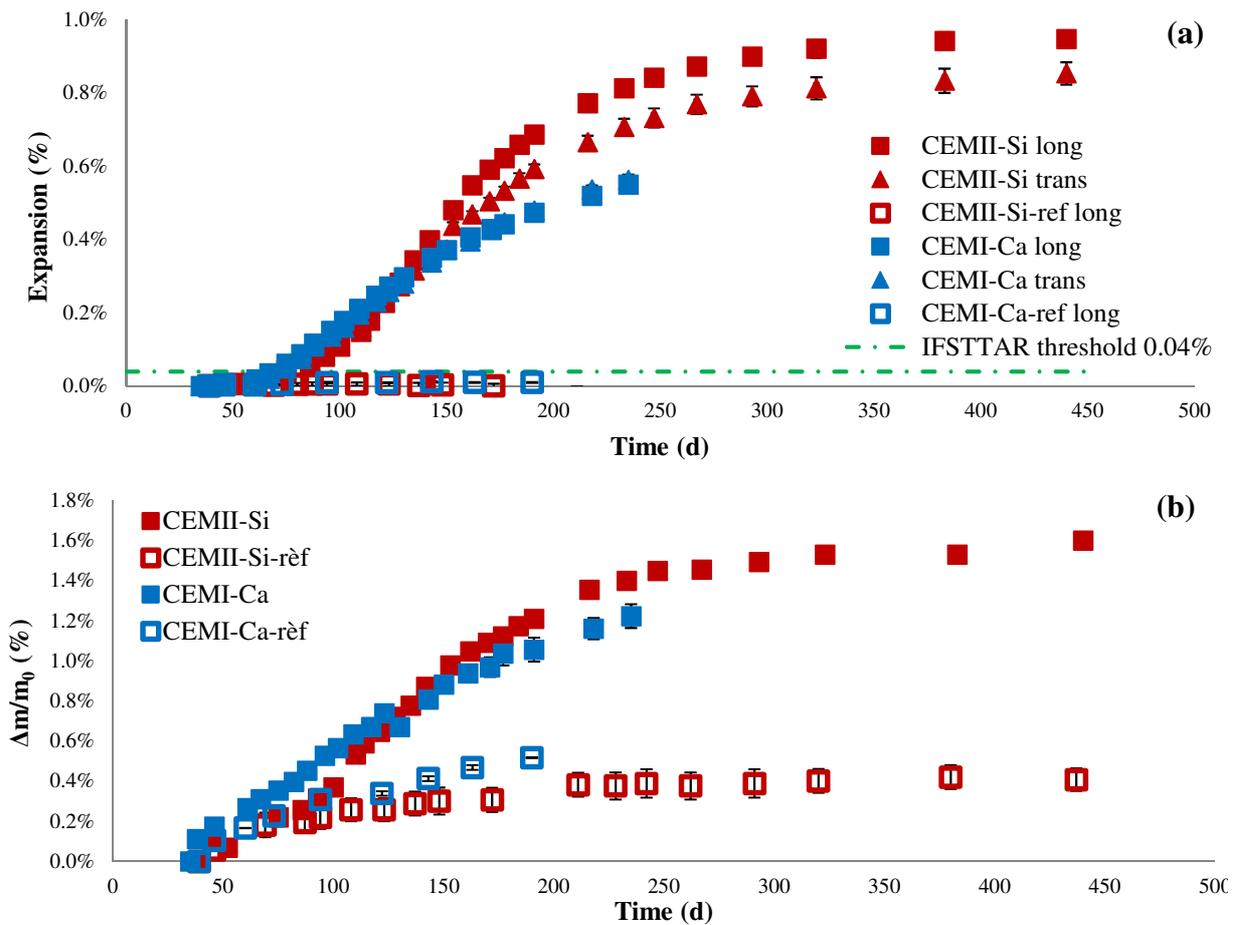
218 Figure 4: Evolution of expansion (transversal and longitudinal) (a) and mass gain (b) versus
