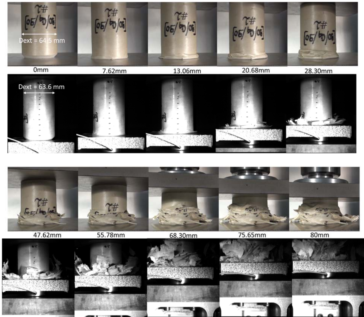
394 Fig. 17: Comparison of the failure scenario between a static and a dynamic tests at iso-displacement 395 [90/0 4 /90] - #2 specimen for static - [90/0 4 /90] - #1 specimen for dynamic.
