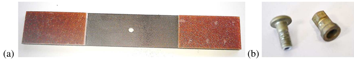
Fig. 2: Open Hole specimen (a) and bolt and nuts used for Filled hole specimens (b).
