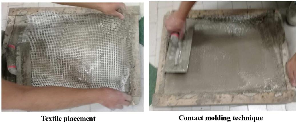
**Figure 1** In-situ hand lay-up technique for PCM-TRC composites
