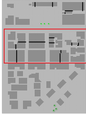
Fig. 5: Sub-model (part of the large model outlined in red) simulated to extract boundary conditions of air temperature and relative humidity.
