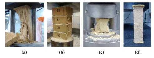
Fig. 2 Compression tests on: (a) vertical entire bricks, (b) 4 stacked half-bricks, (c) mortar aspect ratio 1, (d) mortar aspect ratio 4.
