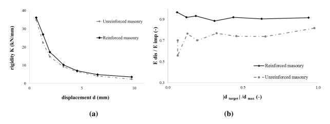
Fig. 11 (a) Stiffness degradation, (b) Energy dissipation.
