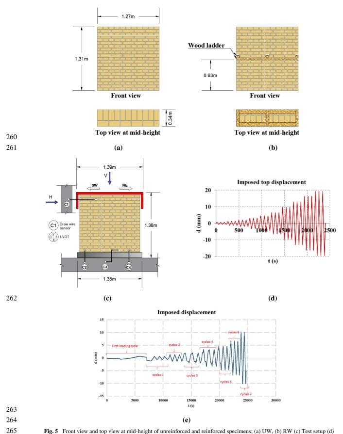
Fig. 5 Front view and top view at mid-height of unreinforced and reinforced specimens; (a) UW, (b) RW (c) Test setup (d)
