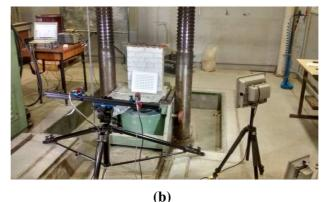
Fig. 3 Compression test on masonry. (a) Position of LVDT captors, (b) Stereoscopique system disposition.
