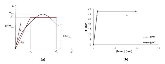
**Fig. 10** Bilinear idealization of the hysteresis envelope: (a) critical parameters on seismic behavior analysis [36] (b) idealization for UW and RW.
