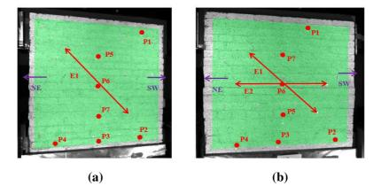
Fig. 6 Reference points and virtual extensometers for; (a) UW, Left, (b) RW, Right.
