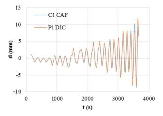
Fig. 7 Virtual CIN and C1 sensor displacement comparison.
