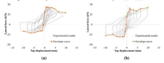
Fig. 9 Hysteresis curves lateral force against displacement for quasi static cyclic tests on: (a) unreinforced masonry shear wall, (b) timber reinforced masonry shear wall.
