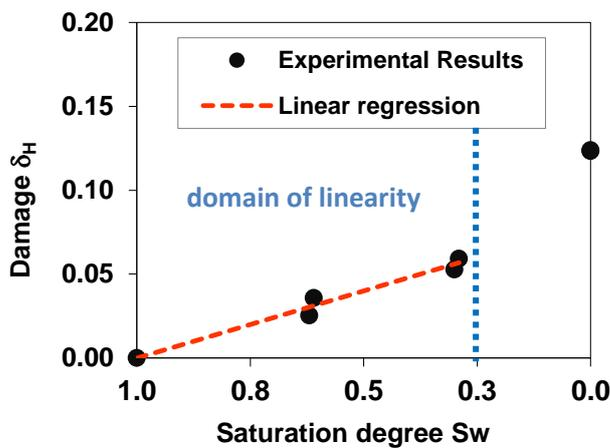
Figure 7. Damage  $\delta_H$  versus saturation degree
