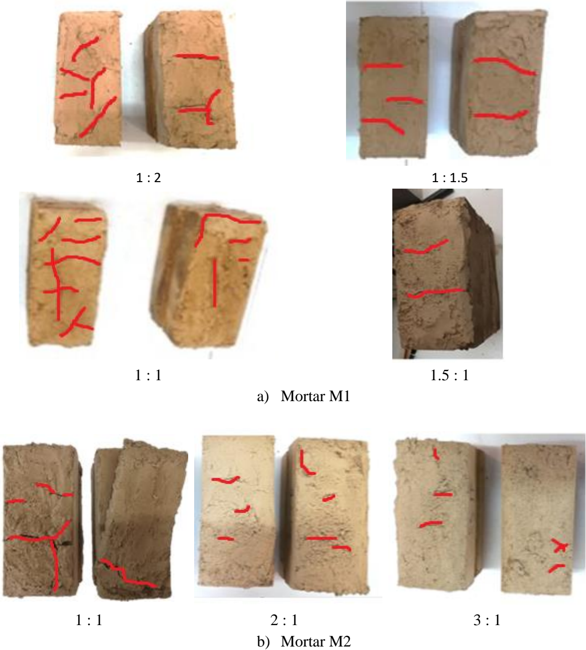
Figure 7: Surface of the assemblies after the drying of mortar for different sand:earth ratios
