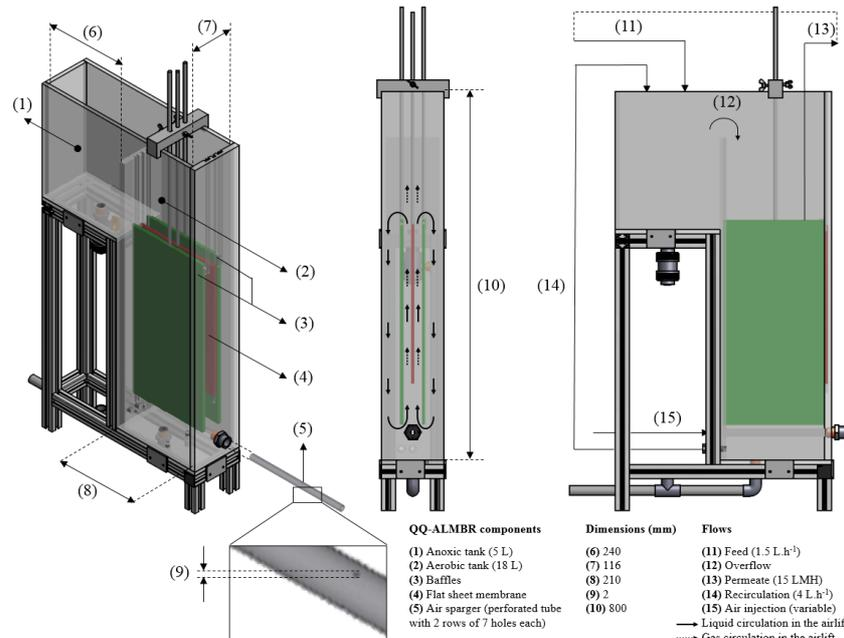
Figure 1 : Diagram of the Quorum Quenching Air-Lift Membrane Bioreactor (QQ-MBR).
