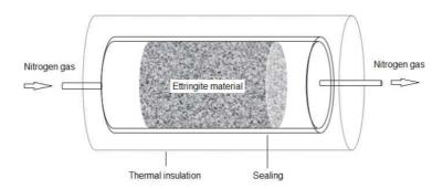
Figure 24: Operating diagram of the second prototype thermochemical reactor
