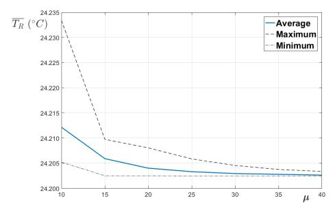
Fig.8: Results of the repeatability test for different values of  $\mu$  ( $R_S = 1$ ,  $R_P = 0.1$  and N = 20) A second test was carried out in order to compare the results obtained with the GA to the ones obtained in section 2.4. This test was run for *N* ranging from 10 to 30 and for  $R_P$  ranging from 0.1 to 0.7. The results are presented in Fig.9.
