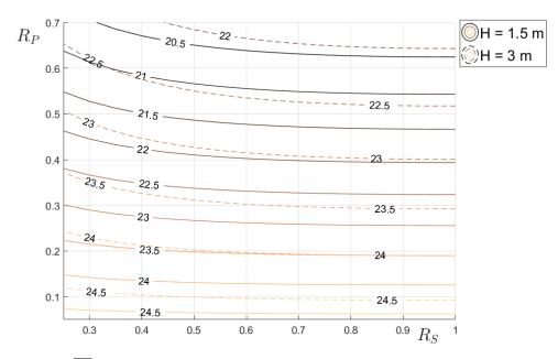
Fig.6: Contours of  $\overline{T_r}$  (in °C) according to  $R_s$  and  $R_P$  for two values of H (full lines: 1.5 m; dashed lines: 3 m)
