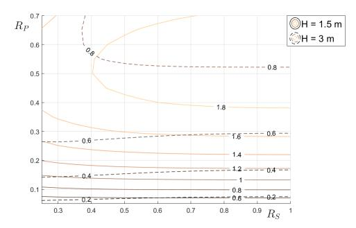
Fig.7: Contours of s (in °C) according to  $R_S$  and  $R_P$  for two values of H (full lines: 1.5 m; dashed lines: 3 m)
