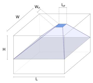
Fig.2: Room equipped with a single SRCP emitting radiation toward the working plane In order to compare different cases, we propose to define two non-dimensional ratios. First,  $R_S$  is defined as in (1) so as to represent the shape of the room. *W* is defined to be always shorter than or equal to *L*, meaning that a square room is considered when  $R_S$  equals one, and a rectangular room when  $R_S$  is less than one.
