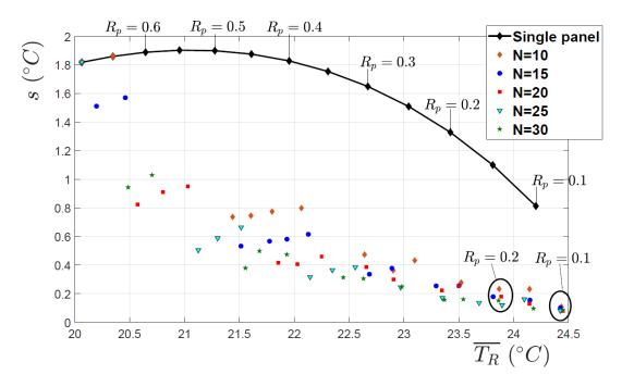
Fig.10: s and  $\overline{T_R}$  values obtained for a single and multiple SRCPs when  $f_2$  is used as the cost function ( $R_s = 1$ )
