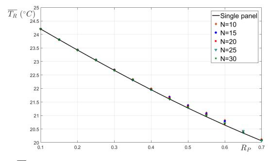
Fig.9: Best  $\overline{T_R}$  values obtained for N panels and for a single panel placed in the middle of the ceiling ( $R_S = 1$ )
