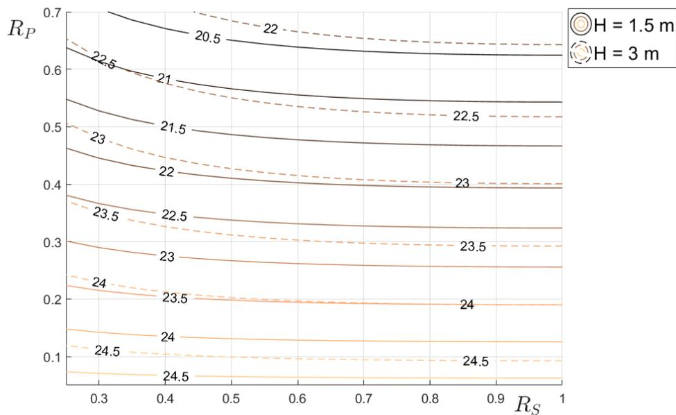
**Fig.6: Contours of  $\bar{T}_r$  (in  $^{\circ}\text{C}$ ) according to  $R_S$  and  $R_P$  for two values of  $H$  (full lines: 1.5 m; dashed lines: 3 m)**
