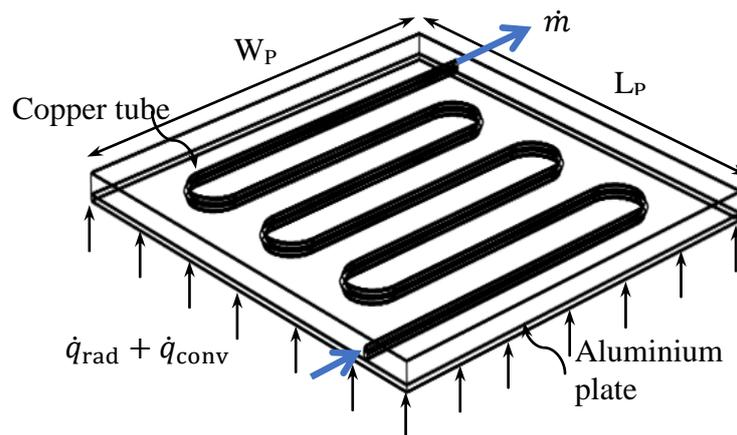
**Fig.1: Scheme of a typical SRCP system made of a copper tube placed above an aluminium plate (adapted from [19])**
