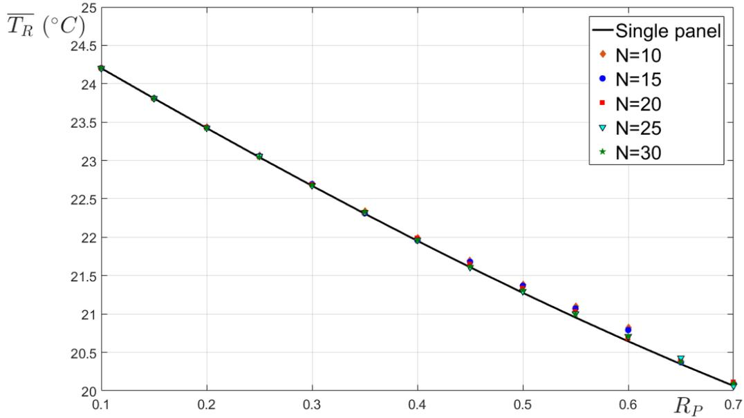
**Fig.9: Best  $\overline{T}_R$  values obtained for  $N$  panels and for a single panel placed in the middle of the ceiling ( $R_S = 1$ )**
