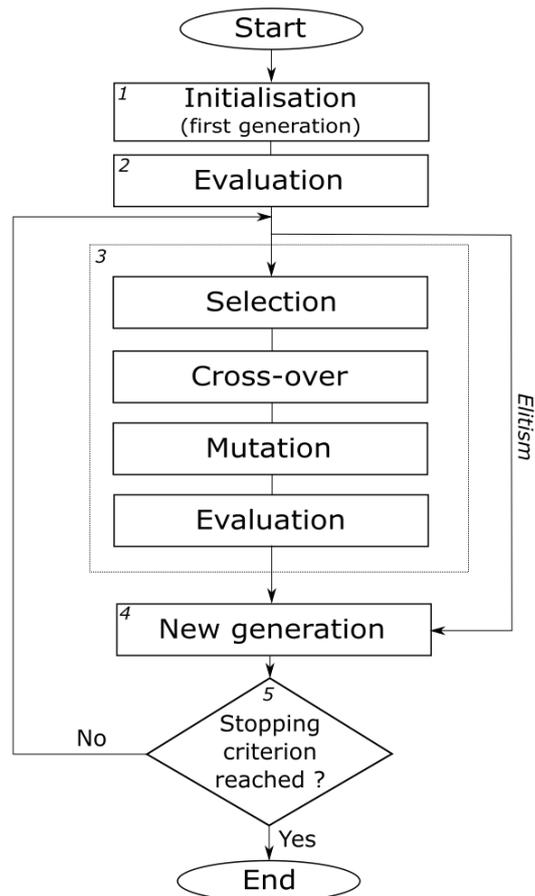
**Fig.4: Flow chart of a generic genetic algorithm**
