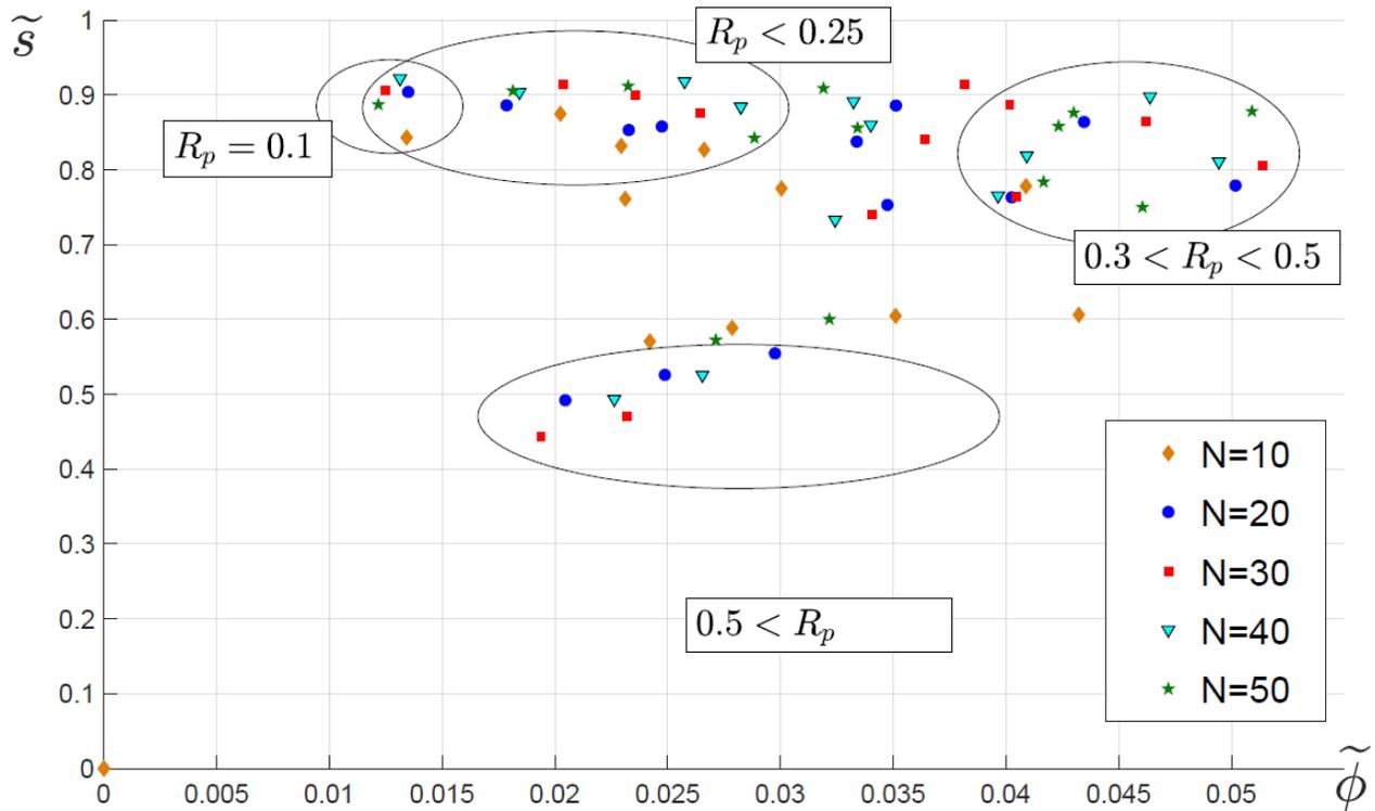
**Fig.11:  $\tilde{s}$  and  $\tilde{\phi}$  obtained when  $f_3$  is used as the cost function for  $R_p$  ranging from 0.1 to 0.7 ( $R_s = 1$ )**
