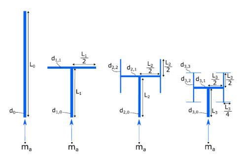
FIGURE 4. Network shape for bifurcation level N ranging from 0 (left, corresponds to the straight pipe) to 3 (right). The overall fluid volume is fixed. The networks are drawn to scale in accordance with the results of Section 3.2.
