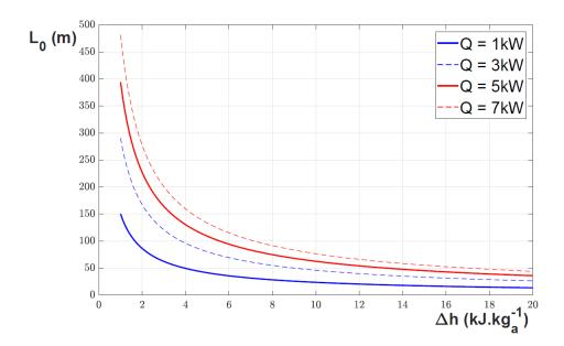
FIGURE 3. Pipe length as a function of the enthalpy difference  $(\Delta h = h_{in} - h_w)$  for different values of the targeted cooling power
