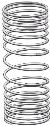
Figure 2: 3D model of variable pitch spring Figure 3: Comparison of theory and simulation
