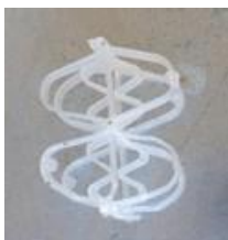
Figure 2 : Raschig Super Ring ® example
