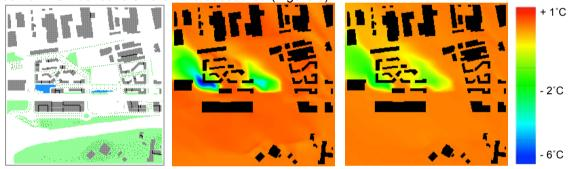
Figure 8: air temperature difference between the "Blue case" and the Base case, during daytime (left) and nighttime (right).
