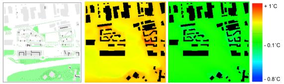
Figure 7: Air temperature difference between the "White case" and the Base case, during daytime (left) and nighttime (right).
