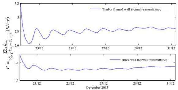
Figure 2: Monitoring of the thermal transmittance of two wall typologies
