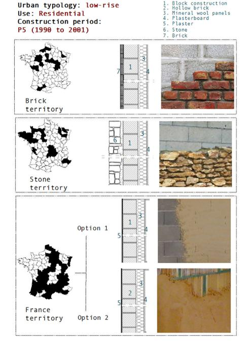
Fig. 5. Constructive system for the walls for the example of low-rise residential buildings of construction period P5. Information is provided on the main material, the internal and external coating as well as the insulation material.
