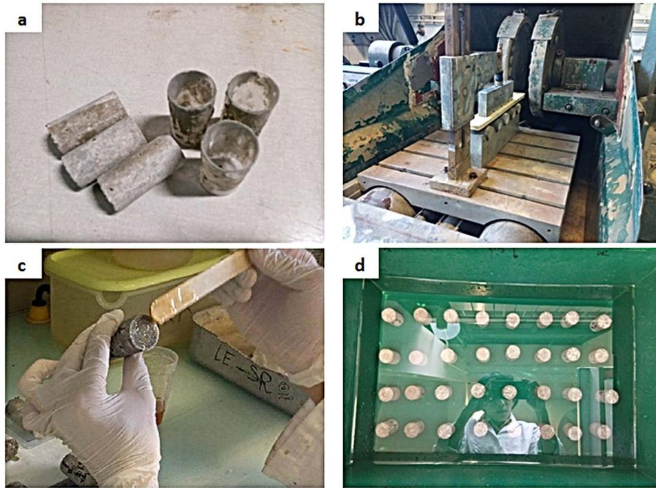
Figure 2: Moulds and specimens (a), grinding specimens (b), coating resin on top and bottom surface of specimens (c), immersing specimens in acid solution (d)
