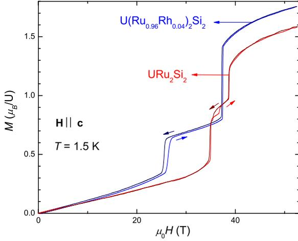
FIG. 1 (color online). Magnetization of  $\text{U}(\text{Ru}_{0.96}\text{Rh}_{0.04})_2\text{Si}_2$  at 1.5 K (blue line). The magnetic field is parallel to the tetragonal  $c$  axis. The magnetization of pure  $\text{URu}_2\text{Si}_2$  is also shown (red line).
