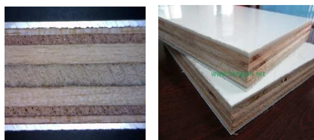
Fig. 3: Allin plywood with aluminium skins.
