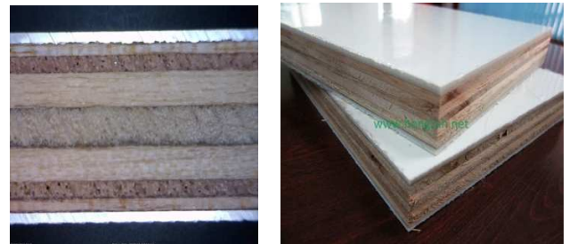
Fig. 3: Allin plywood with aluminium skins.
