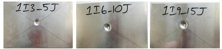
Fig. 6: Plywood with aluminum skins impact pattern.
