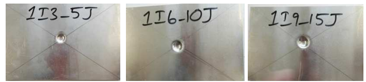
Fig. 6: Plywood with aluminum skins impact pattern.
