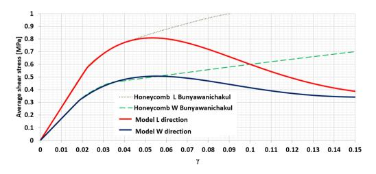
**Figure 3.** Comparison of the experimental Bunyawanichakul's curves [10] and the curves used as reference for this research.
