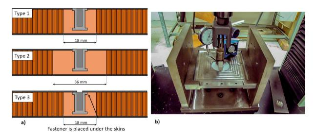
**Figure 1.** Insert's description of type 1, 2, 3 and testing set up. [10]
