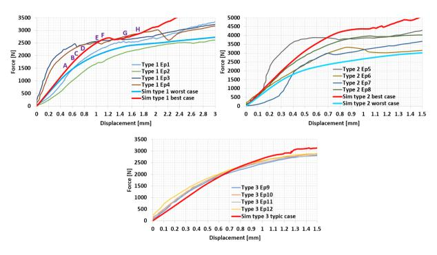
**Figure 7.** Comparison of the experimental and numerical behavior of the loading curves for the inserts type 1, 2 and 3.
