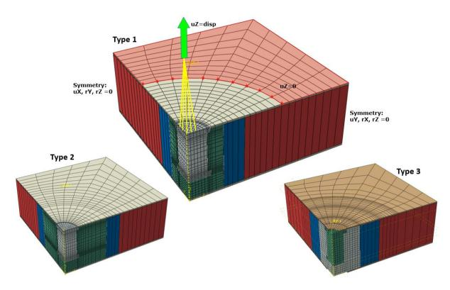
Figure 2. Reduced F.E. models of inserts type 1, 2 and 3.
