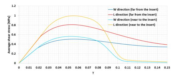
**Figure 4.** Behavior laws of the honeycomb far and near to the insert. (based in [9])
