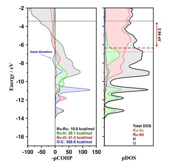
**Fig. 10** Projected DOS and COHP profiles for  $Ru_{55}H_{33}(CH_3COO)_{16}$ ( $2^{COO,H}$ ). Dashed red line and dotted red line on the pDOS profile: *d*-band center ( $\bar{\epsilon}_d$ ) of the 44 surface Ru atoms and of the 11 core Ru atoms, respectively; brown horizontal line: Fermi energy. The energies reported on the pCOHP graph are the IpCOHP indexes (see definition and references in the methods section).
