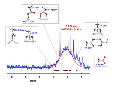
**Fig. 2** Diffusion-filtered <sup>1</sup>H NMR spectrum of  $Ru_x(CH_3COOH)_{0.4y}$  NPs dispersed in THF- $d^8$  at r.t. The broad signal at *ca.* 2.08 ppm was fitted with a Gaussian shape. The DFT <sup>1</sup>H NMR chemical shifts of the methyl group in various models ((CH<sub>3</sub>COOH)<sub>2</sub>, CH<sub>3</sub>COO<sup>-</sup>, [Ru<sub>6</sub>] clusters) are also given. The DFT results are summarized by the burgundy horizontal lines.
