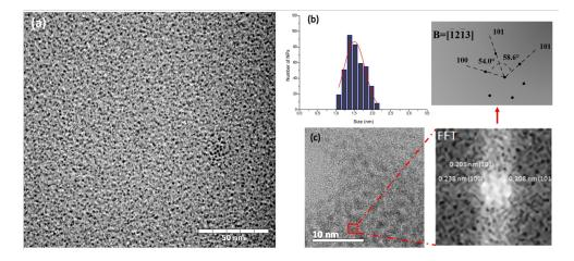
Fig. 1 TEM image and corresponding size histogram of  $Ru_x(CH_3COOH)_{0.4y}$  NPs (a, b); HRTEM image of  $Ru_x(CH_3COOH)_{0.4y}$  NPs with FFT results (c).
