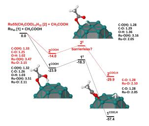
**Fig. 5** Energy profile of the O-H bond dissociation. Black profile and energies: O-H activation on the bare  $Ru_{55}$  NP (model 1); red profile and energies: O-H activation on the  $Ru_{55}(CH_3COO)_{15}H_{32}$  NP (model 2). For the sake of clarity, geometries are shown for the bare case only; very similar geometries are found in model 2. Energies are given in kcal.mol<sup>-1</sup>. Some characteristic bond lengths are also given, in Å (same color convention as the energy profiles).
