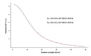
**Fig. 3** Diffusional attenuation of the 1.90 - 2.20 ppm area for  $Ru_x(CH_3COOH)_{0.4y}$  NPs dispersed in THF- $d^8$  at r.t. Data were analysed with a bi-exponential least-square fitting.
