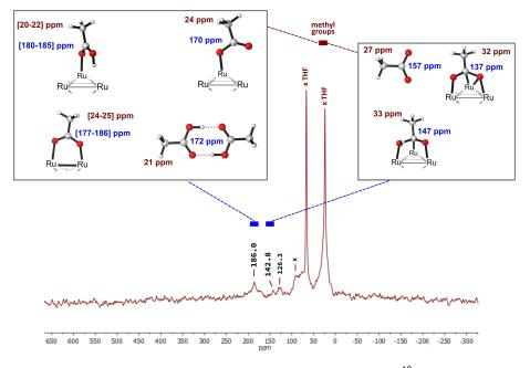
Fig. 6 <sup>13</sup>C CP Hahn-MAS NMR of Ru<sub>x</sub>(CH<sub>3</sub>COOH)<sub>0.4y</sub> NPs dispersed in mesoporous silica. DFT <sup>13</sup>C NMR chemical shifts of the acid group and carboxylate in various models. Blue: carboxyl group, burgundy: methyl group.
