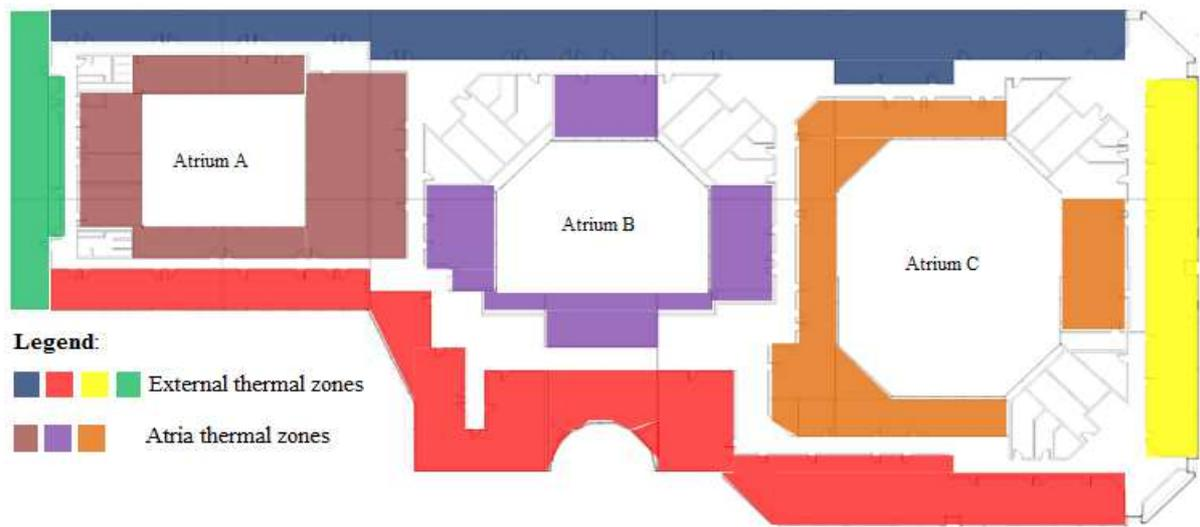
**Figure 9.** Thermal zones under consideration for the calculation of the cooling load
