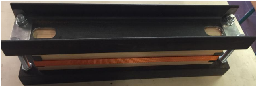
Figure 4: Clamping equipment for the ultrasonic measurements
