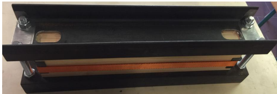
Figure 4: Clamping equipment for the ultrasonic measurements
