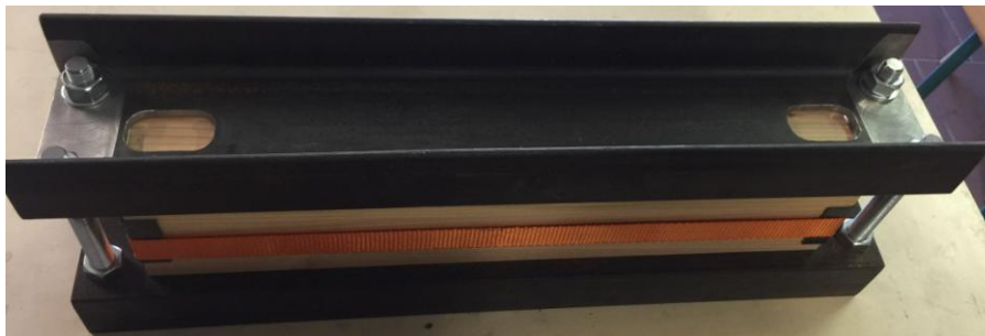
Figure 4: Clamping equipment for the ultrasonic measurements
