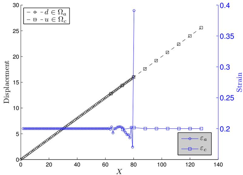
**Fig. 11** Displacement and strain plots versus position for the non-local, interpolated coupling, with 2 elements per  $\Omega^b$  ( $ES = 1/15$ ).
