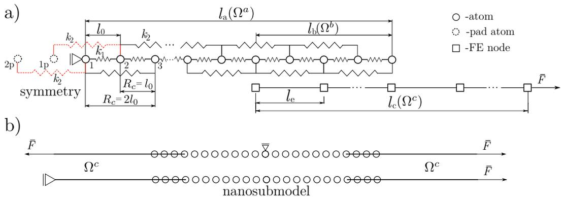
**Fig. 2** 1D coupling model scheme with the symmetry BC on the left end of the atomistic domain a). The utilization of the symmetry BC yields the configuration equivalent to the nSM inserted into the continuum chain b).
