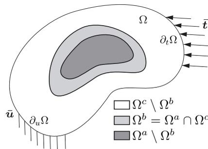
**Fig. 1** Scheme of the coupled model and the nSM technique.
