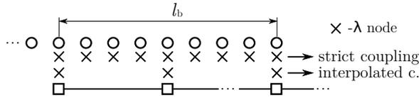
**Fig. 4** Scheme of the distribution of the LM nodes for strict and interpolated coupling.
