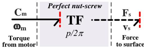
FIGURE 6. FUNCTIONAL MODEL OF MPT IN BOND-GRAPH.
