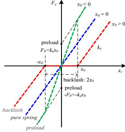
FIGURE 9. ELASTIC CHARACTERISTIC OF PROPOSED COMPLIANCE MODEL.
