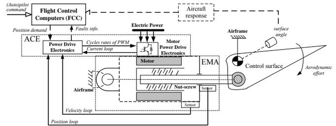
**FIGURE 1. SCHEMATIC STRUCTURE OF AN EMA ACTUATION SYSTEM.**
