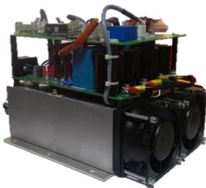
Fig. 3 : DC/AC (one phase) converter prototype
