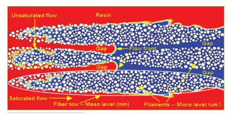
Fig. 2: Simulation of resin flow in a 3D reinforcement at different scales
