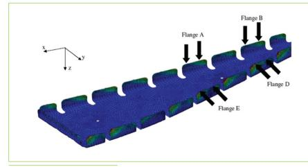
Fig. 5: A350 rib spring-back computation
