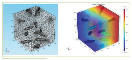
Fig. 3: Modelling thermal conductivity in a doped composite material
