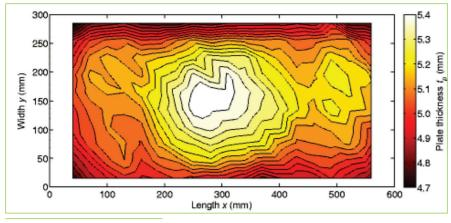
Fig. 4: Example of ply thickness spatial evolution
