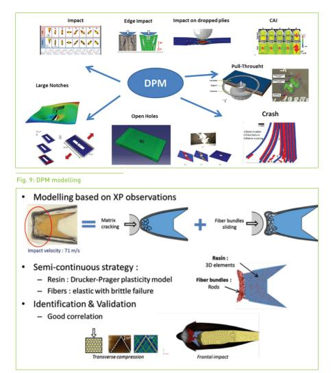
Fig. 10: Semi-continuous modelling for frontal impact of rotor blades
