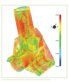
Fig. 8: Simulation of short fibre injection in a complex part (aircraft fitting)
