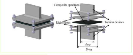
Fig. 13: Edge ring crack torsion test (ERCT)
