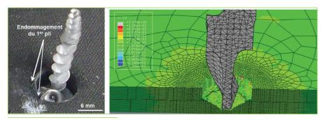
Fig. 7: Chip formation analysis (left) during CFRP/Ti multi-material drilling (simulation on the right)
