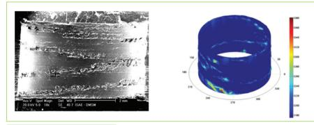
Fig. 6: Hole roughness analysis to define drilling quality indicators
