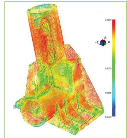
Fig. 8: Simulation of short fibre injection in a complex part (aircraft fitting)
