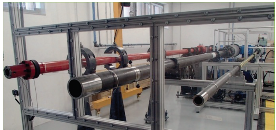
Fig. 14: STIMPACT platform gas guns
