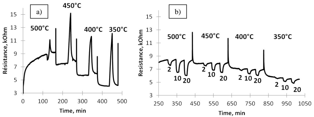
Figure 1. Sensor response to (a) NO<sub>2</sub> (1 ppm) and (b) CO (2, 10, 20 ppm) at different temperatures.
