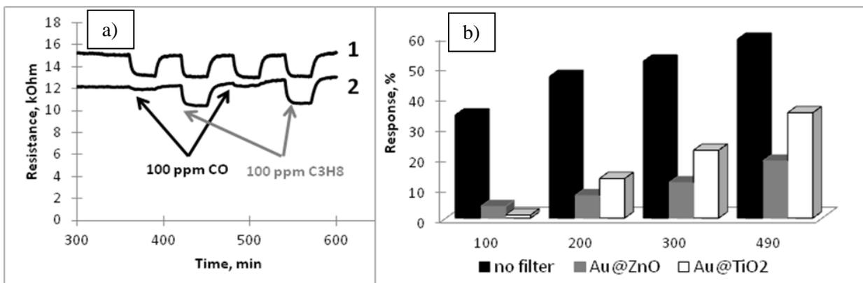
Figure 3. a) SnO<sub>2</sub> sensor response towards 100 ppm CO and C<sub>3</sub>H<sub>8</sub> in the absence (1) and presence (2) of Au@ZnO filter, b) comparison of sensor response towards CO at different concentrations in the presence of Au@ZnO or Au@TiO<sub>2</sub> filters.
