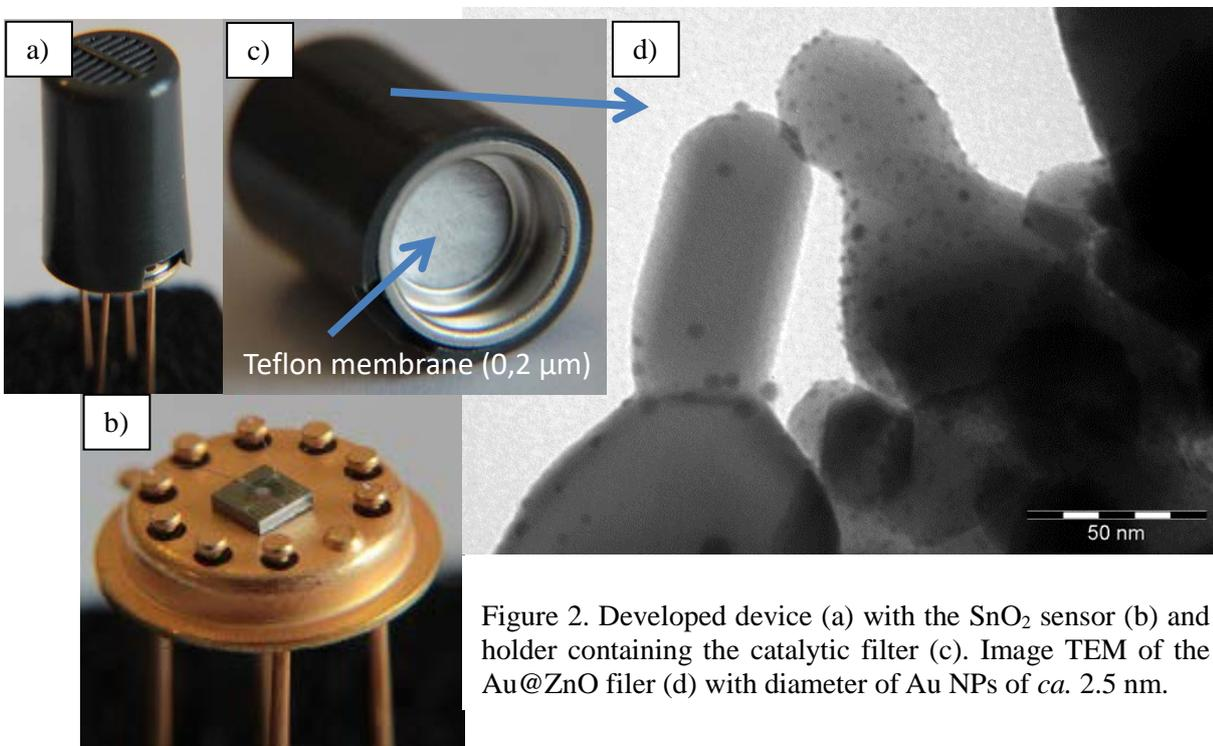
Figure 2. Developed device (a) with the SnO<sub>2</sub> sensor (b) and holder containing the catalytic filter (c). Image TEM of the Au@ZnO filer (d) with diameter of Au NPs of *ca.* 2.5 nm.
