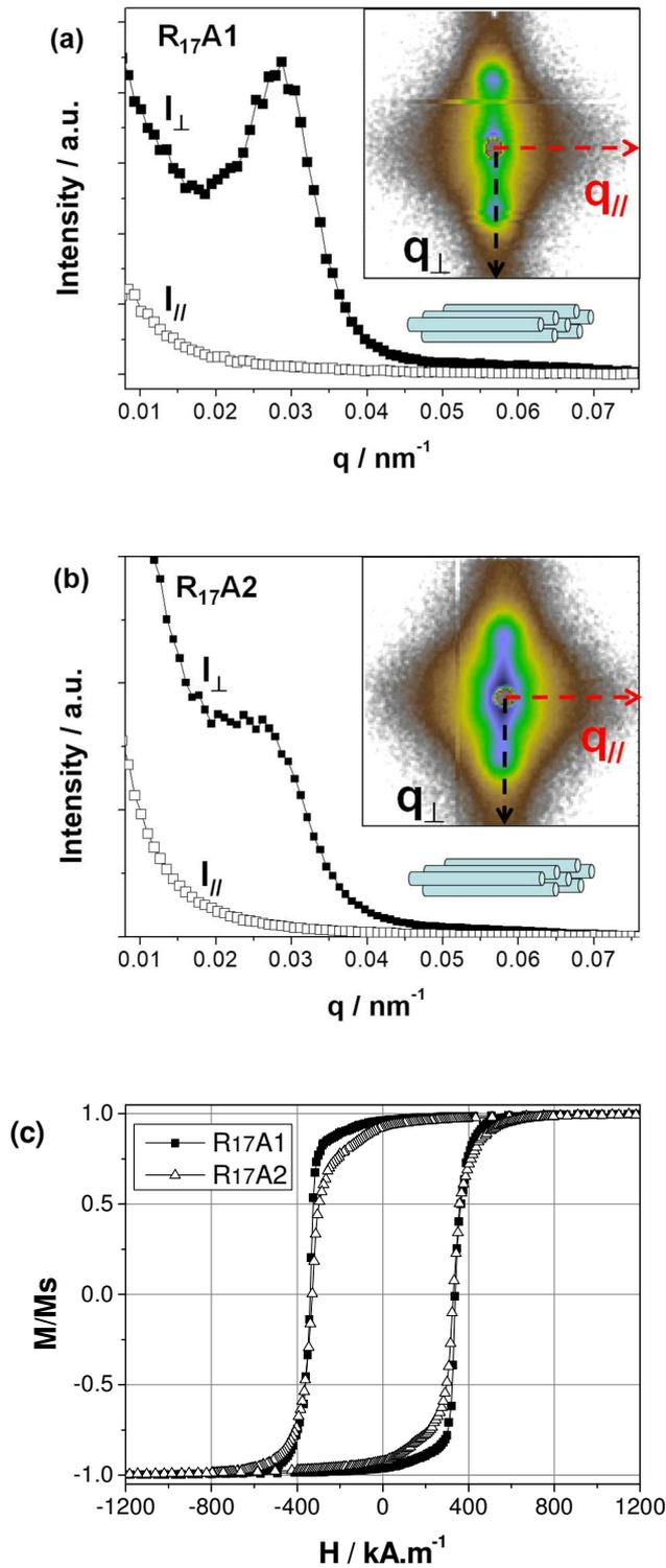
**Fig. 2** (a) and (b) Small angle neutron intensity profile scattered by two cobalt nanorod assemblies (R<sub>17</sub>A1 and R<sub>17</sub>A2), perpendicular (black square) and parallel (open square) to the rod alignment. *Inset*: corresponding 2D SANS pattern; (c) Magnetization curves in parallel configuration of the assemblies R<sub>17</sub>A1 (black square) and R<sub>17</sub>A2 (open triangle).
