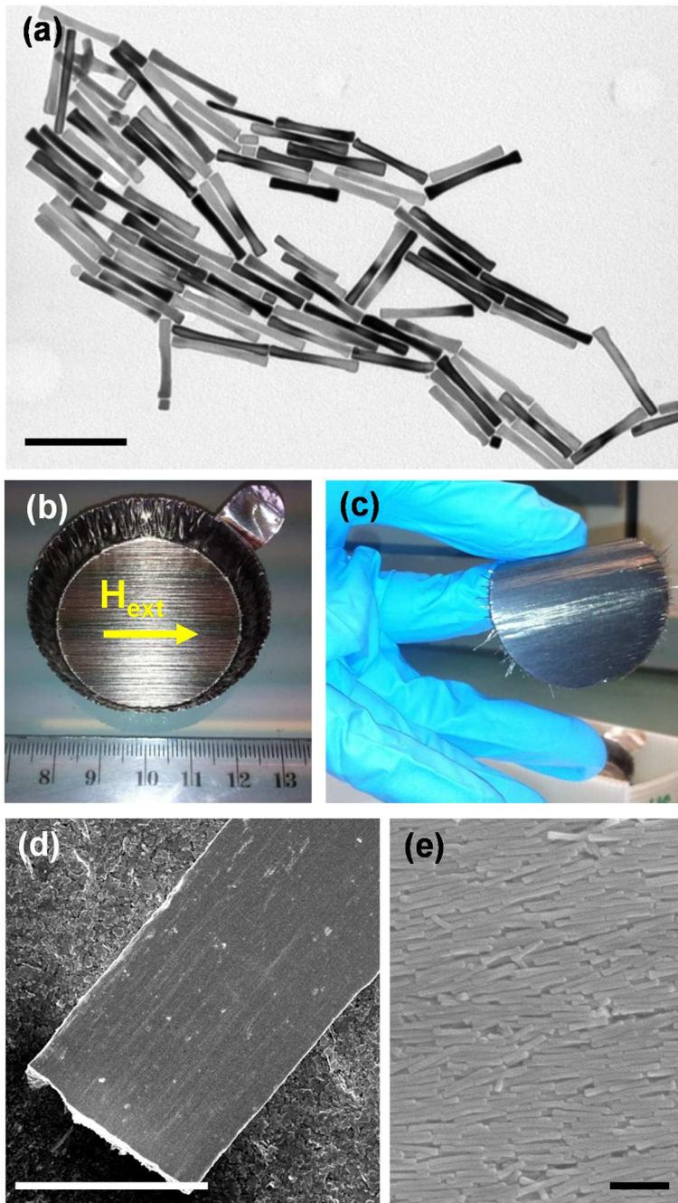
**Fig. 1** (a) TEM image of cobalt nanorods prepared by the polyol process prior to their alignment ; (b) and (c) wafer of cobalt nanorods obtained by drying a suspension in chloroform under an external magnetic field of 1T; (d) SEM image of a millimeter size parallelepiped made of aligned cobalt nanorods; (e) SEM image of the surface of a parallelepiped. Scale bars denote (a) 200 nm, (d) 100  $\mu$ m and (e) 200 nm.
