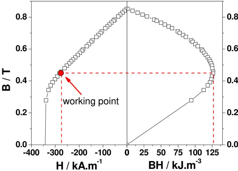
**Fig. 3** Second quadrant of the B-H loop and energy product  $(BH)_{max} = 125 \text{ kJ.m}^{-3}$  of the Co NR assembly R<sub>22</sub>A1.
