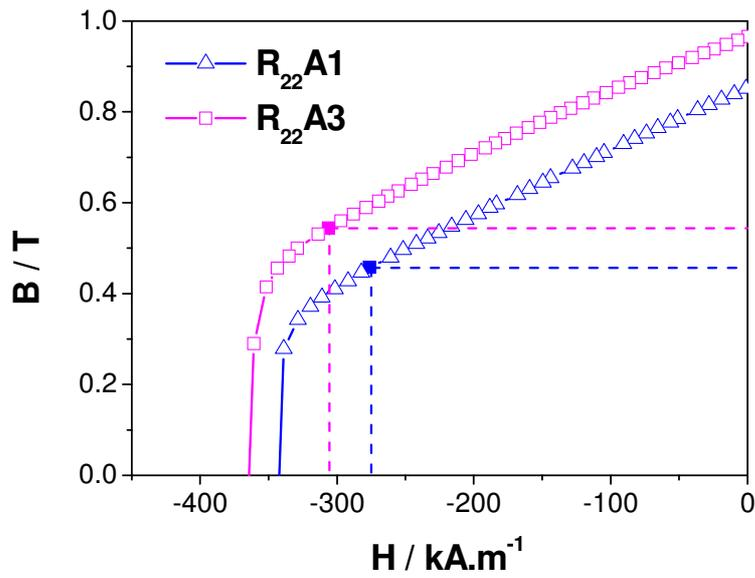
**Fig. 5** Second quadrant of the  $B(H)$  loops and working points of the assemblies  $R_{22}A1$  and  $R_{22}A3$  prepared with cobalt nanorods of mean diameter  $d_m = 22$  nm. Sample  $R_{22}A1$  (blue triangle):  $V_M = 48.7\%$ ,  $SQ = 0.93$ ,  $(BH)_{max} = 125 \text{ kJ.m}^{-3}$ ; sample  $R_{22}A3$  (magenta square):  $V_M = 54.4\%$ ,  $SQ = 0.96$ ,  $(BH)_{max} = 165 \text{ kJ.m}^{-3}$ .
