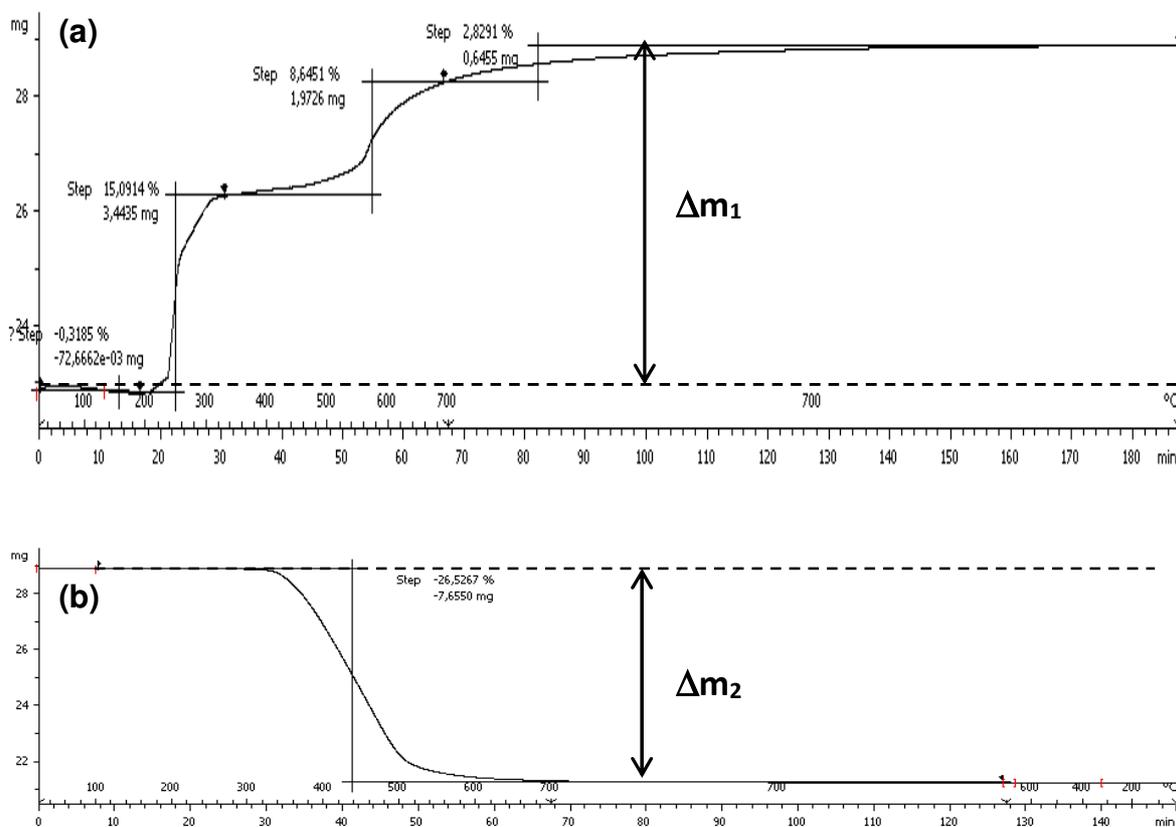
**Fig. S2** Thermogravimetric analysis of  $m_0 = 22.8$  mg of the sample R<sub>31</sub>A4 (a) oxidation in air up to 700°C associated with a mass gain  $\Delta m_1 = +5.99$  mg followed by (b) reduction at 700°C in H<sub>2</sub>/Ar = 4/96 atmosphere associated with the mass loss  $\Delta m_2 = -7.65$  mg. The cobalt mass fraction in this sample is  $\%w(Co_{total}) = (m_0 + \Delta m_1 + \Delta m_2)/m_0 = 92.7\%$
