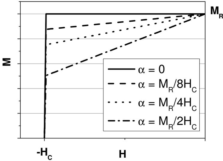
**Fig. 6** Second quadrant of model  $M(H)$  loops with  $M = M_R + \alpha \times H$  for different value of the slope  $\alpha$ . The squareness of the four loops is 1, 0.9375, 0.875 and 0.75.
