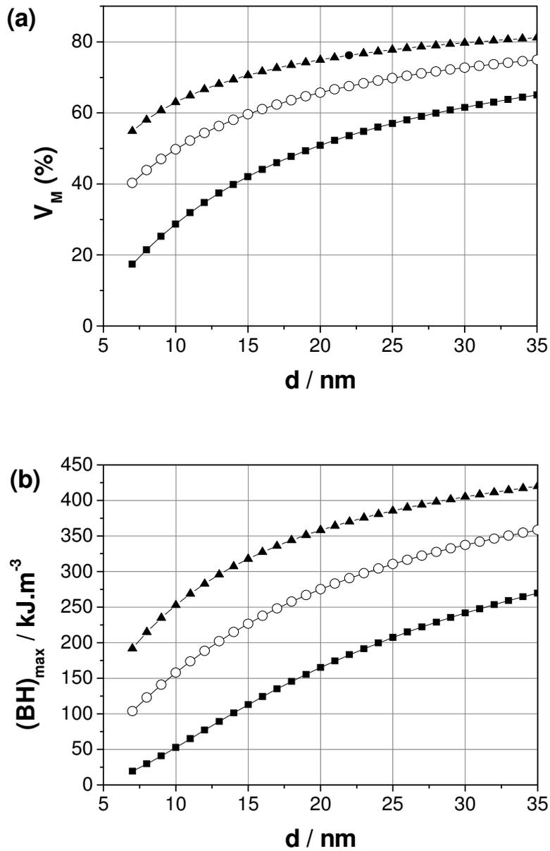
**Fig. 8** Magnetic volume fraction (a) and energy product (b) of perfectly aligned hexagonal arrays of cobalt nanorods of mean diameter  $d$  separated by a ligand shell of 3.5 nm, oxidized rods with a CoO shell thickness of 1.2 nm (full square) and non-oxidized rods (open circle); non oxidized rods separated by a ligand shell of 2 nm (full triangle).
